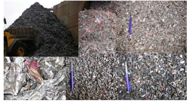
Figure 7: Diverse properties of recycling materials (in which clockwise: steel from 1153 ELV's; Cu fraction; Al/Mg/Cu/Zn fraction; plastic fraction; Al/Mg/Cu/Zn fraction; steel fraction)
