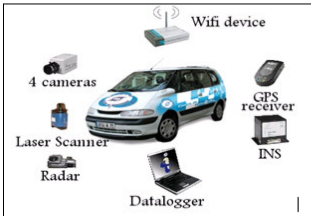
Figure 1: The first LARA prototype (Renault Espace car) with its sensors.
