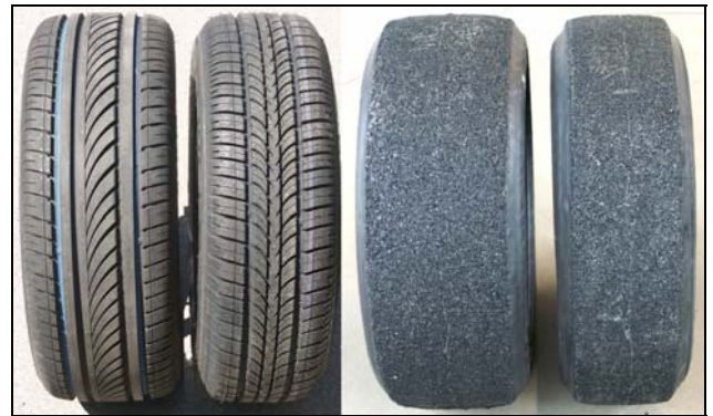
Fig. 4. Two porous tread tyre prototypes together with the regular tyres used as carcasses for the porous tread (after buffing-off the existing tread).
