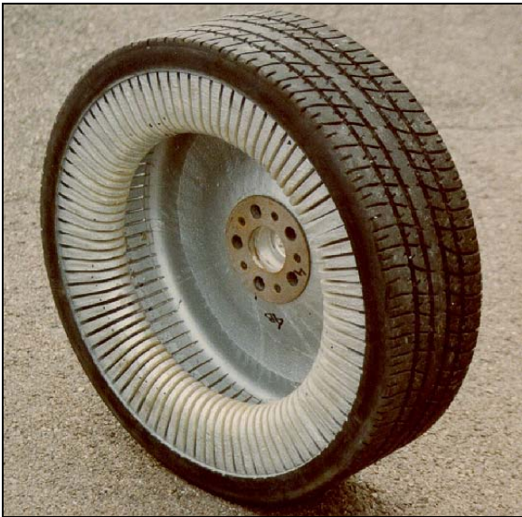
Fig. 3. Composite wheel, invented by Mr H. E. Hansson, tested by VTI in 1991, see Table 25.1 in [Sandberg & Ejsmont, 2002]. The Michelin Airless tyre somewhat resembles this design.
