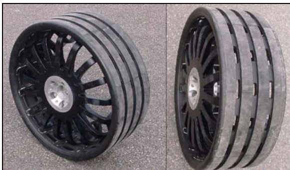
Fig. 1. Early version of a composite wheel (not a good design re. noise). Note the ventilation holes in the tread. New version is underway in which the spokes are much better designed to reduce stiffness variations around the circumference and with better distributed ventilation holes.
