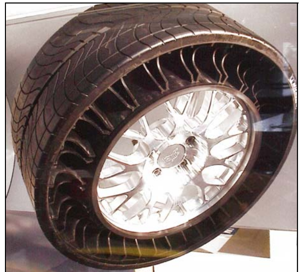
Fig. 2. The TWEEL as it was presented the first time at the motor show in Detroit in January 2005. Photo kindly supplied by Dr Lin Kung, Kumho Tires, USA.
